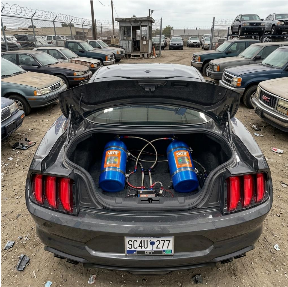
Exhibit #4 Image of trunk mounted Nitrous Oxide Systems canisters in Vance Mustang
